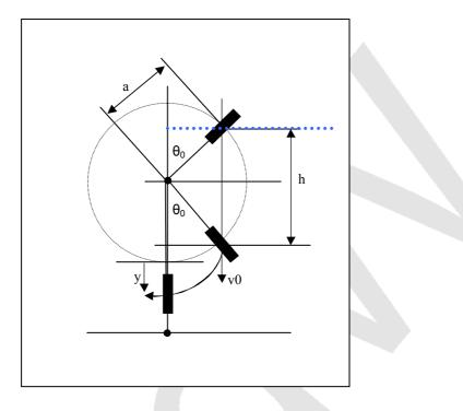
**Fig.8:** The geometry of the pendulum fall. Instead of  $\theta_0=0$  (straight fall) there is now  $\theta_0>0$ . The length of the rope above the last bolt is  $a = \frac{h}{2\cos(\theta_0)}$ . The blue dotted line is the line of impact forces of equal size.
