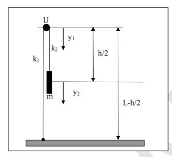
**Fig. 3:** The same fall situation as in Fig. 1 with additional spring constants  $k_1$  and  $k_2$  left and right of the deflection U.  $y_1$  is the shift of a small rope element under an applied force with U as reference point.
