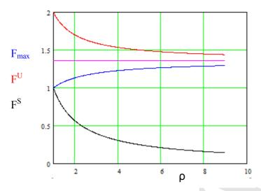
**Fig.6:** While the external friction  $\rho$  makes the fall  $F_{max}$  harder for the falling climber (blue curve), the force  $F^{s}$  on the belayer (black) and the force  $F^{U}$  on the last clipped bolt (red) become smaller. The straight line (magenta) is the limiting case of fall factor f = 2. All falls are normalized to  $F_{max}$  without friction.
