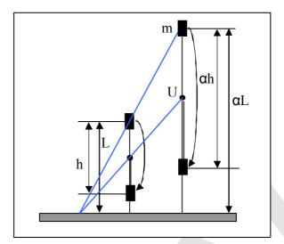
**Fig. 2:** Scale invariance of the impact force: All falls, where the mass m and the position of the last runner U lie on arbitrary superposed points on the blue lines, have the same fall factor and thus the same impact force.
