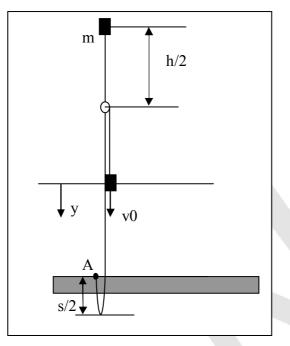
**Fig. 1:** A straight fall where the mass m falls a distance h and has the velocity  $v_0$  at y=0. At this point the rope (with length L and fixed at A) begins to stretch when there is no rope slack (s=0).
