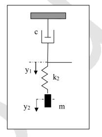
**Fig.7:** Maxwell model with a spring  $k_2$  and a viscous element c.
