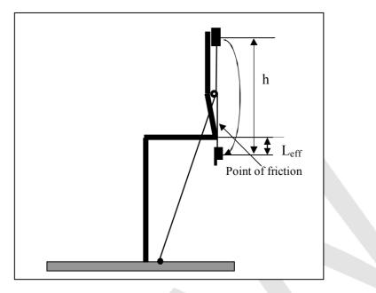
Fig.5: Fall over a roof edge. With external friction fall factors greater than 2 are possible, because for a fall height h  $L_{eff}$  can become smaller than h/2.
