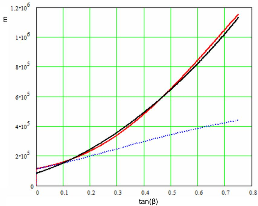
**Fig.5:** Energy consumption  $E$  [J] when walking uphill as a function of the gradient  $\tan(\beta)$  for the model (9,16) (black curve) compared with [11] (red curve) and the energy consumption for an efficiency 1 (dashed blue line).
