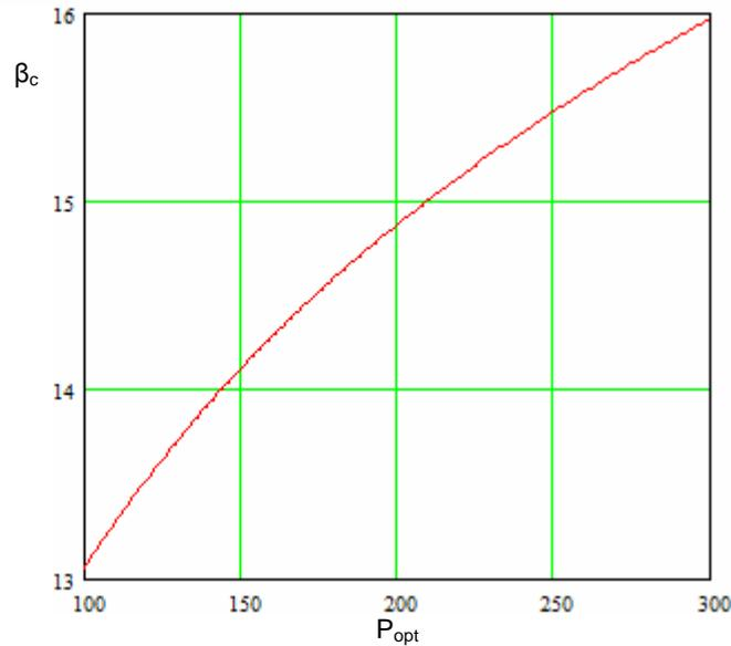
**Fig. 11:** Critical gradient angle (17) in degrees as a function of the power parameter  $P_{opt}$ .
