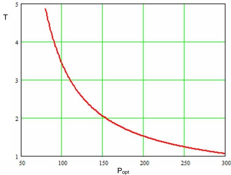
Fig.4: Walking time T of eq. (9) in hours as a function  $P_{opt}[W]$ . With  $h=1000m$  and  $L=4000m$  a typical situation was chosen.
